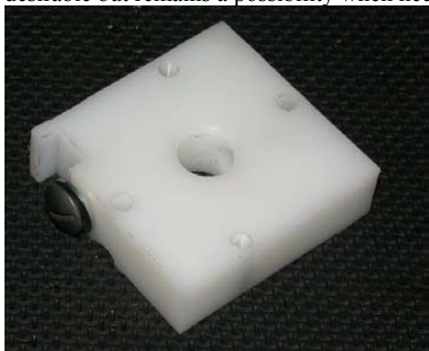
This nylon spacer has tapped holes to attach to case and countersunk through holes to mount new movement. (The calibration potentiometer discussed later is shown in the photograph to the right connected to the blue/brown wires).
