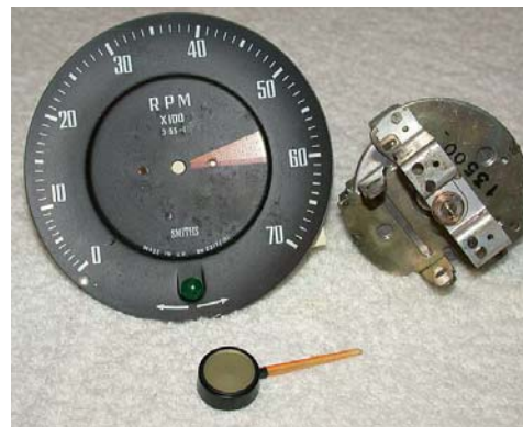
Removing needle and disassembled gauge.
