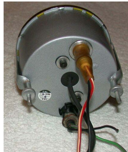
Completed conversion. Cosmetically restored with electronic movement inside.
