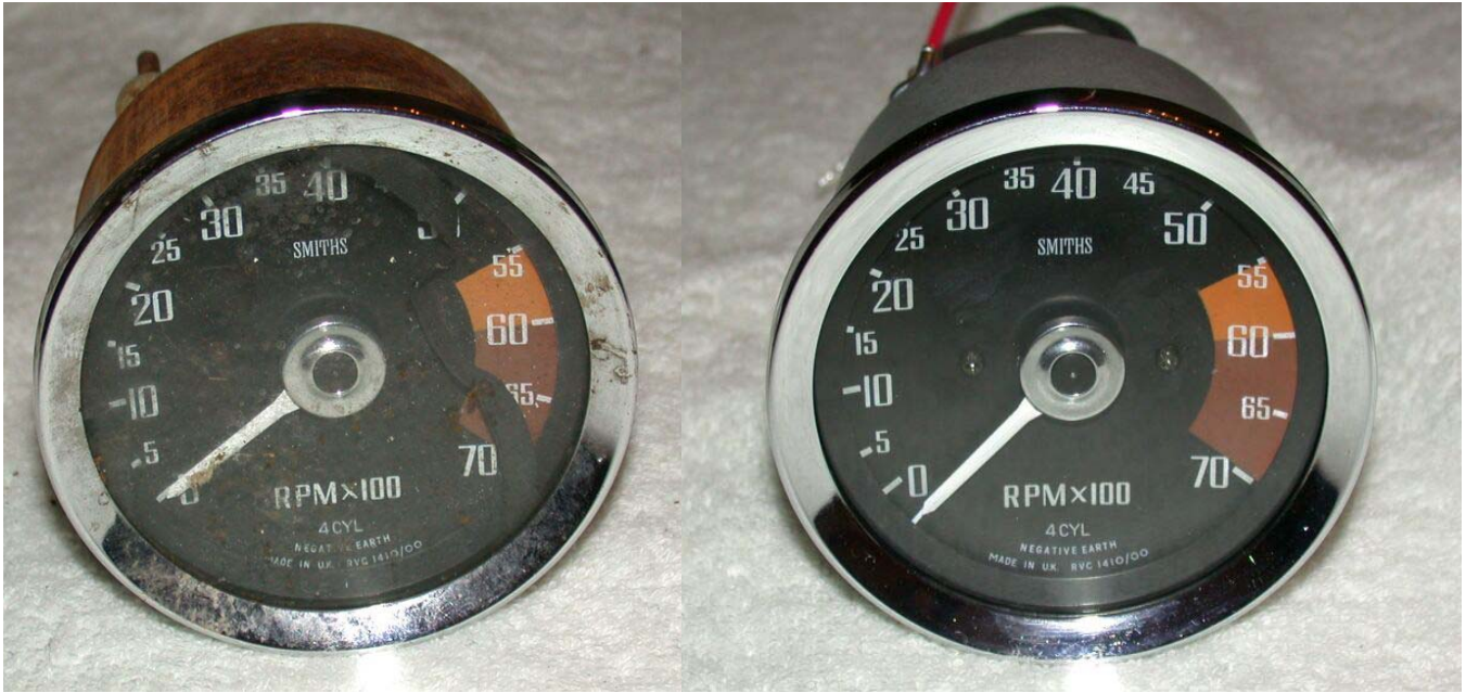
Smiths RVC Tachometer before and after conversion and cosmetic restoration.
