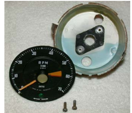
Left to Right: Smiths gauge with the bezel, front glass, and reflector removed. Back of gauge & fillister screws. Smiths gauge with the movement removed and rubber mounting isolator seen inside.
