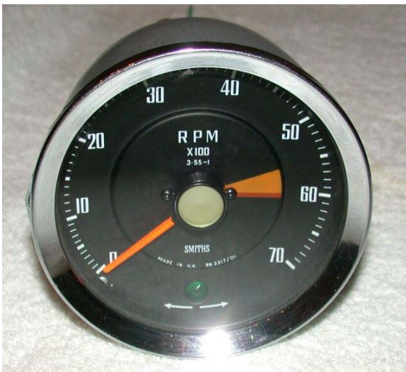
Completed conversion. Cosmetically restored with electronic movement inside.
