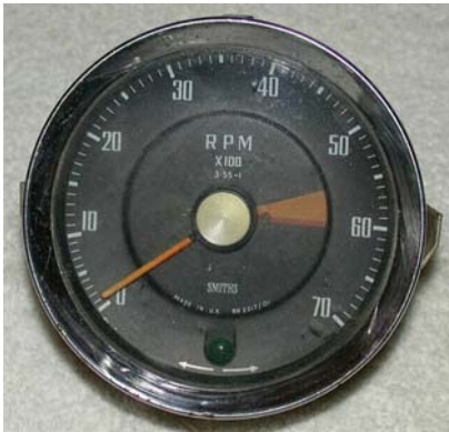
This Smiths mechanical tachometer will be converted to an electronic movement.
