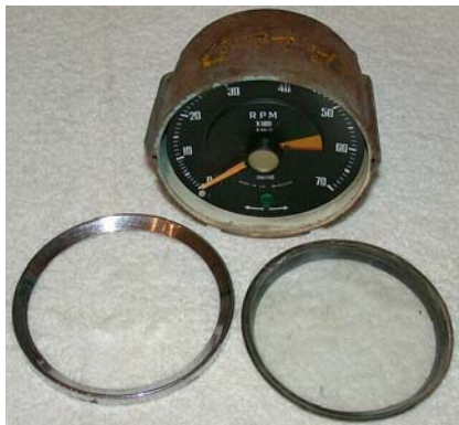
Left to Right: Smiths gauge with the bezel, front glass, and reflector removed. Back of gauge & fillister screws. Smiths gauge with the movement removed and rubber mounting isolator seen inside.
