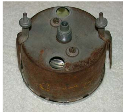
This Smiths mechanical tachometer will be converted to an electronic movement.
