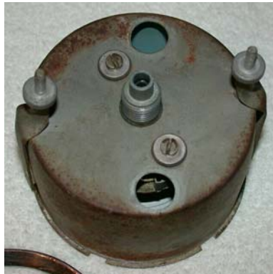
Left to Right: Smiths gauge with the bezel, front glass, and reflector removed. Back of gauge & fillister screws. Smiths gauge with the movement removed and rubber mounting isolator seen inside.
