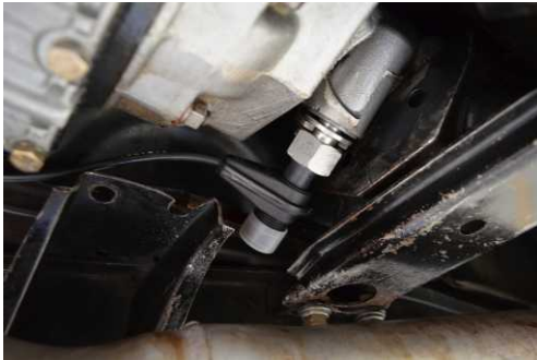
Under the car, the old angle-drive mechanism was removed and replaced with the digital sender
