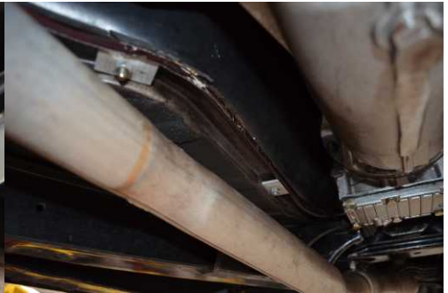
The cable was routed along the frame up to the cabin following the route of the original cable
