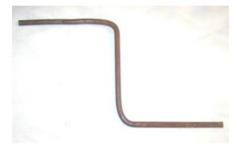
The stay under the glove box, the glove box, and the right side ventilation and demister ducts are removed. The rubber grommet in the hole through which the temperature control and choke cables pass is pushed forward into the engine compartment. The tool is then inserted into this hole beside the cables; see next photo.
