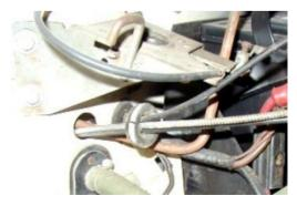
The hood is released by pushing the bottom of the tool to the left causing it to rotate around the middle segment and the top to move to the right and pressing against the hood release lever.
