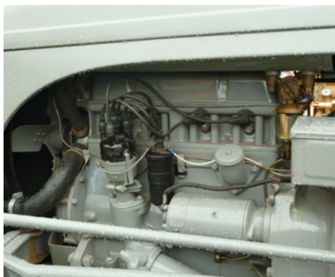
Spark plug side of cylinder head, showing the valve pushrod tubes (Ferguson TE20 tractor)
